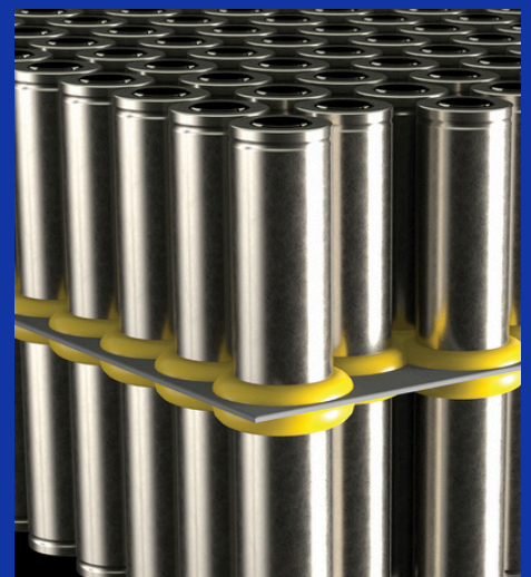
Figure 4. Example of thermally conductive adhesives bonding cylindrical cells to a cold plate
