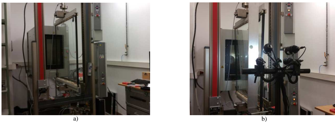
Fig. 20 Test assembly for the torsion tests with 1 000 mm x 1 000 mm IGUs; a) no load applied; b) moment of force = 200 Nm
