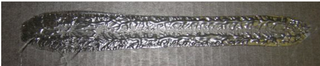
Joint Disrupted / Opened While Still a Hot Liquid
