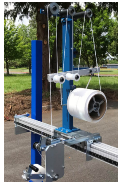
Dry End Tape applicator shown on a support stand.
